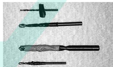
Please insert the prepared drill carefully into the appropriate spot on the rail. In order to avoid the aluminium borders being damaged, **do not activate the drilling machine** until the **drill bit is in the piper rail**. All sinkings have to be accomplished according to the usual practice.
